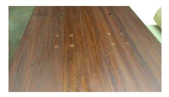
**Tensioned models** : Your board has been conceived with a specific pen-hole connection (visible by the 8 times 4 pins on the surface) which will allow the board to set. The surface is made out of 3 shelf that are primarily connected with this pen-hole technique. To ease the manufacturing process we also apply minor glue to keep the shelf together while proceeding with the pen-hole assembly. Once assembled the glue has no function anymore.
