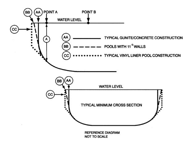
Figure 2- Typical pool design configurations
