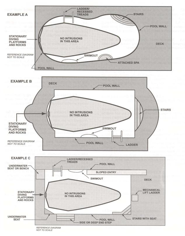
Figure 6- Top view examples of accessory equipment and pool features prohibited in the water envelope
