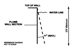
Figure 1- Maximum allowable wall slope
